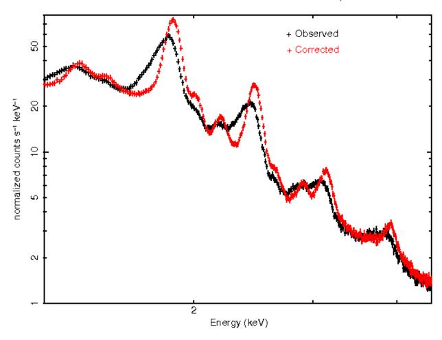
Figure C.7: Comparison of the observed and the trap corrected spectra extracted from WT observations of the Cas A SNR in October of 2007. The fit of the Silicon K $\alpha$  line with an asymmetric Gaussian in IDL yielded a FWHM of  $152 \pm 13$  eV for the observed spectrum and of  $106 \pm 3$  eV for the corrected spectrum.
