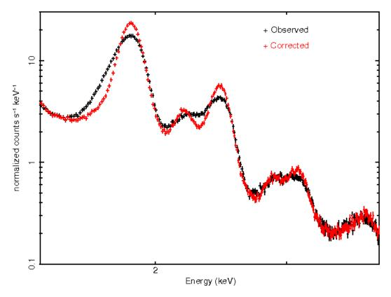
Figure C.6: Comparison of the observed and the trap corrected spectra extracted from a PC mode observation of the Tycho SNR from October 2009. The fit of the Silicon K $\alpha$  line with an asymmetric Gaussian in IDL yielded a FWHM of  $179\pm8$  eV for the observed spectrum and of  $132\pm3$  eV for the corrected spectrum.
