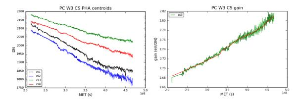
Figure 2: Swift-XRT CCD measurements from the corner source data at a CCD temperature of  $-60^{\circ}C$  from 2007-Sep-05 to 2015-Nov-01. The left panel shows the measured  $^{55}$ Fe line centroids from the four corner sources. The right panel shows the gain coefficient (GC0\_TRAP) estimated using equation A.11 and used for trap-corrected spectra (in green the measured monthly averaged gain values, in red the modelled gain evolution with time). Error bars are  $1\sigma$  estimates.
