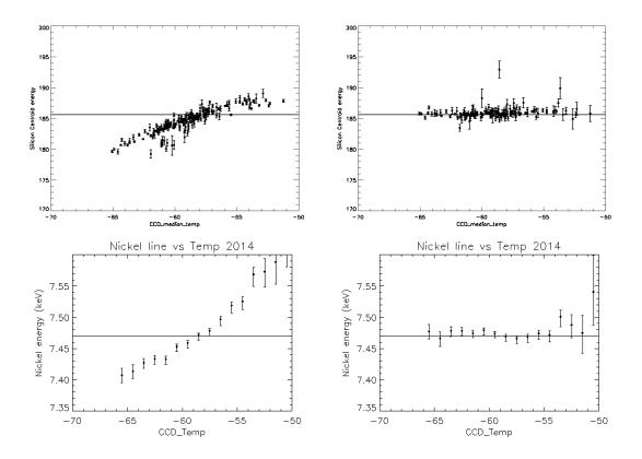
Figure C.9: The Tycho Silicon line (top left panel) and the instrumental Nickel K $\alpha$  line (bottom left panel), in the data from the 2014-2015 cmpaign, show evidence of energy shifts from the expected values as a function of temperature. Processing the PC data with the updated gain file, that includes temperature dependent trap tables, the Gaussian fits in both cases give energies close to the expected values at all temperatures, as can be seen in the right panels.
