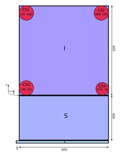
Figure A.1: Schematic of the Swift-XRT CCD22 identifying the imaging (I) and frame-store (S) sections, the readout register (R), and the  $^{55}$ Fe corner sources (CS). Charged is clocked in the parallel direction (Y), through both the imaging and frame-store sections, which have charge transfer inefficiencies  $CTI_{p,i}$  and  $CTI_{p,f}$ , respectively, and in the serial direction through the readout register with  $CTI_s$ .
