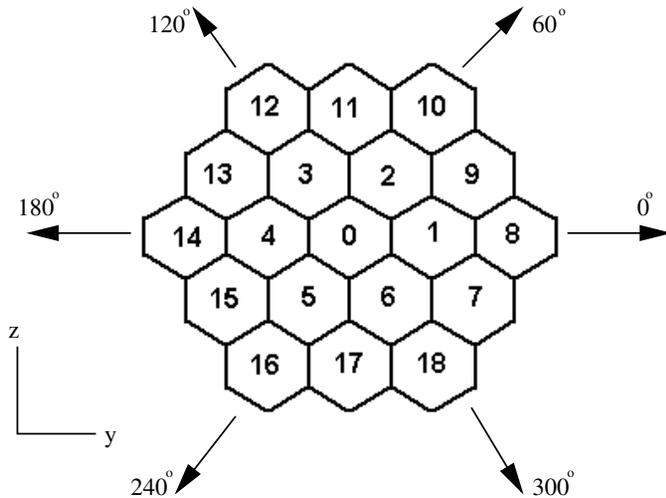
Coincidence events between adjacent Ge detectors define azimuthal distribution.
