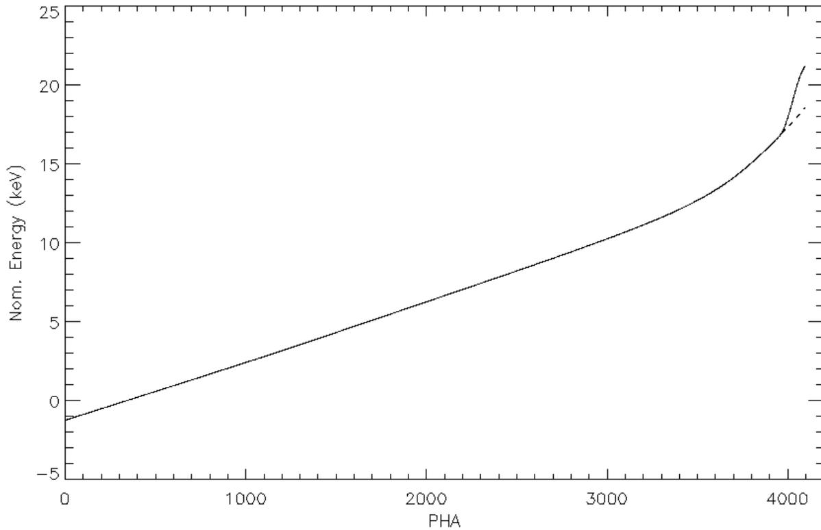
**Figure 1.** Approximate energy to channel relation for NICER DET\_ID 50. The optmv7 (old) solution is solid; the optmv7e (new) solution is dashed.
