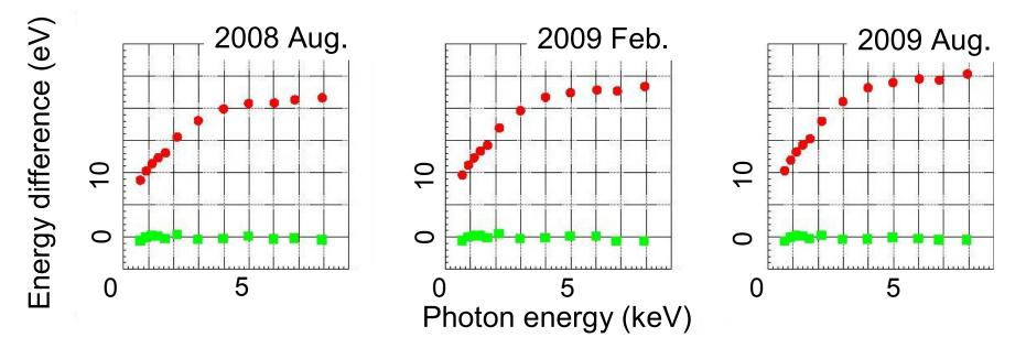
The difference in photon energy between the 2x2 mode and the standard 5x5 (or 3x3) modes as a function of photon energy. Red and green points show those with previous and new CALDBs.
