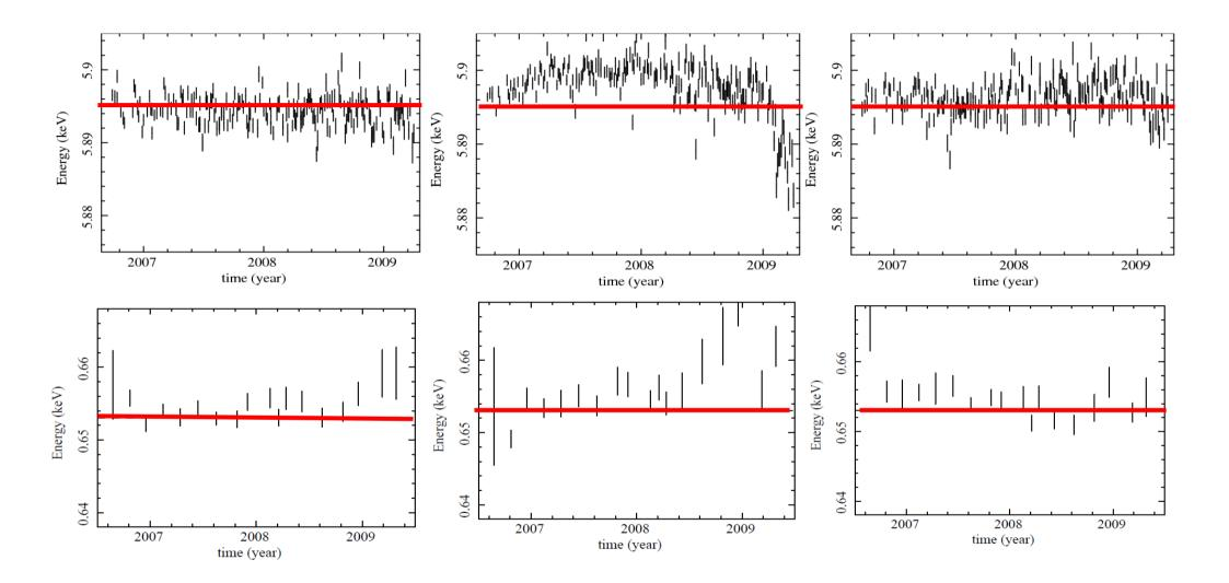
The center energies of the Mn I K  $\alpha$  (55Fe cal. source) and O VIII K  $\alpha$  (SNR E0102) lines determined with ae\_xi[0-3]\_makepi20090615.fits. The red lines show the theoretical values.
