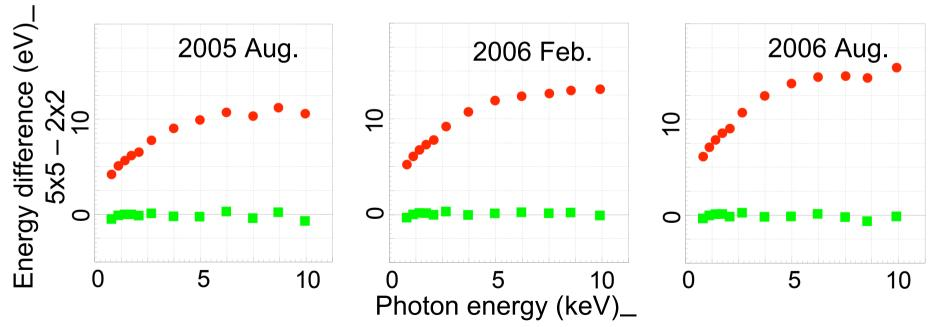
The difference in photon energy between the 2x2 mode and the standard 5x5 (or 3x3) modes as a function of photon energy. Red and green points show those with previous and new CALDBs.
