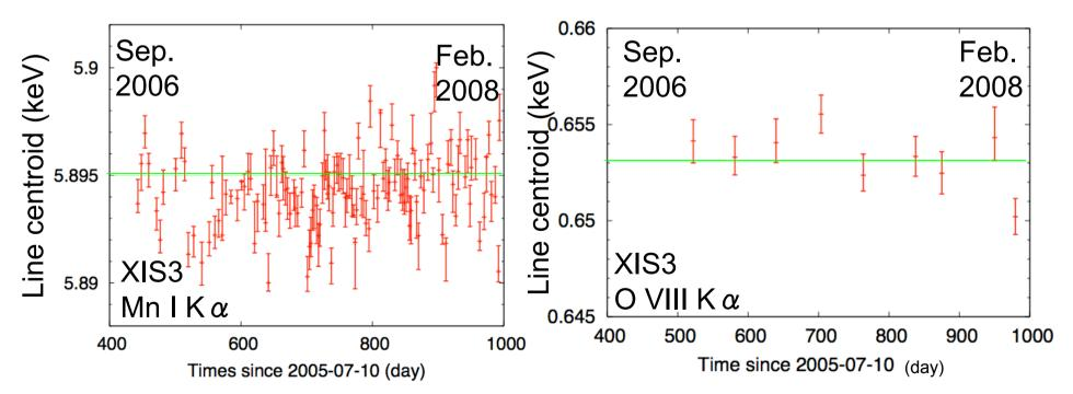
The center energies of the Mn I K  $\alpha$  (cal source) and O VIII K  $\alpha$  (E0102) lines determined with ae\_xi[0-3]\_makepi20080825.fits. The green lines show the theoretical values.
