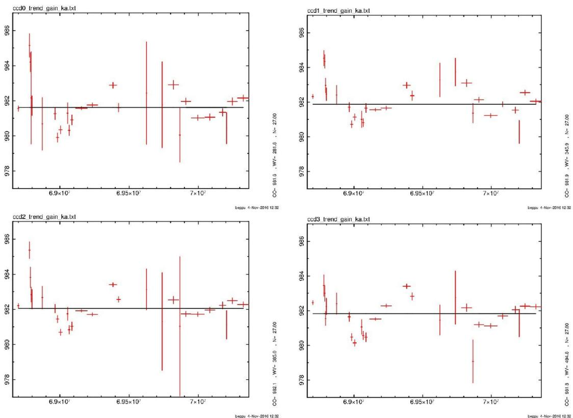
Fig.3-1 Time history of peak value of 55Fe data taken in CCD1 (top left), 2(top right), 3(bottom left) and 4(bottom right) after adopting the CALDB parameters. The uncertainty of  $\sim 12$  eV at 5.9 keV was found.
