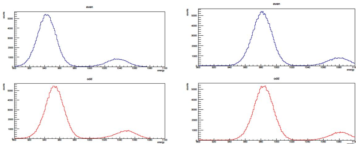
Fig.2-4 (left): Grade 0 spectra of  $^{55}\text{Fe}$  data taken with CCD1CD before even/odd correction. Top and bottom figures show the even and odd column data, respectively. Individual even/odd gains were measured (left) and corrected (right) segment by segment.
