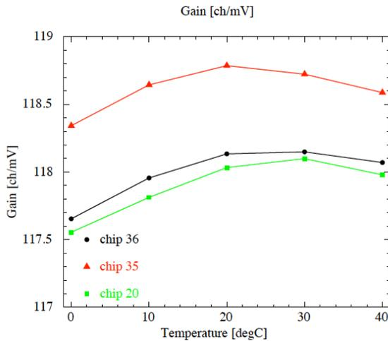
Figure 2-3 shows temperature dependences of video gain, which show a loose peak around 20-30 degree Celsius and individual characteristic.
