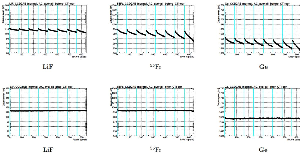
Fig.2-2 a) Top and b) bottom figures show a PH of each line as a function of the number of transfer before and after CTI correction, respectively. Before correction, so-called saw-tooth shape is seen due to periodic charge-injection (CI) technique. Blue vertical lines indicate CI rows.
