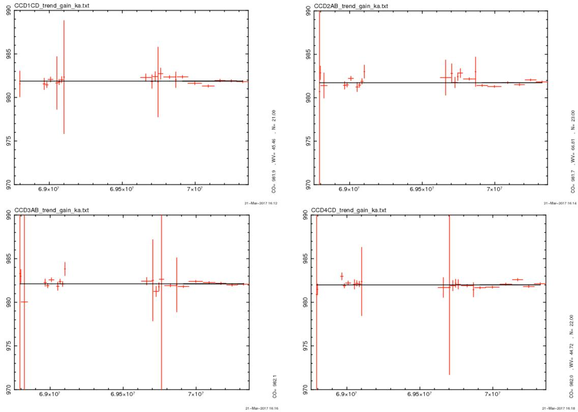
Fig.4-1 Time history of peak value of <sup>55</sup>Fe data (PI) taken in CCD1 (top left), 2(top right), 3(bottom left) and 4(bottom right) after the gain correction.
