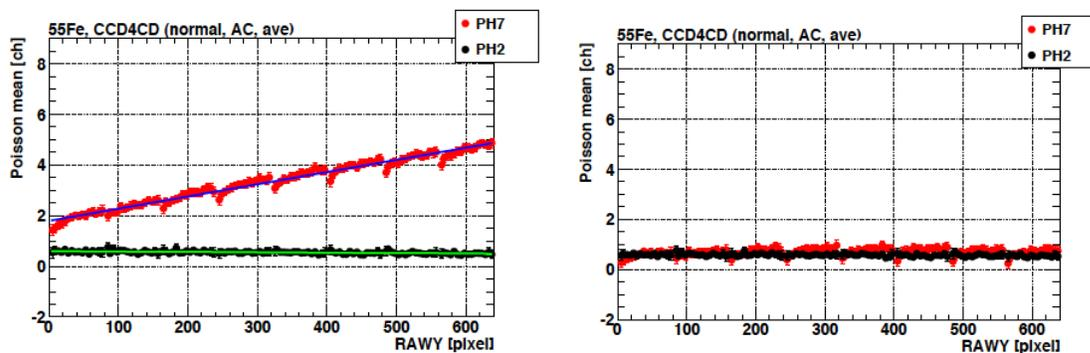
Fig.2-1 Left figure shows PHs of preceding (black) and succeeding (red) pixels of Fe-55 events. PHs of succeeding pixels are shifted to positive due to the charge trail as a function of the number of transfer. Right figure shows the same plot as shown in left but after trail correction
