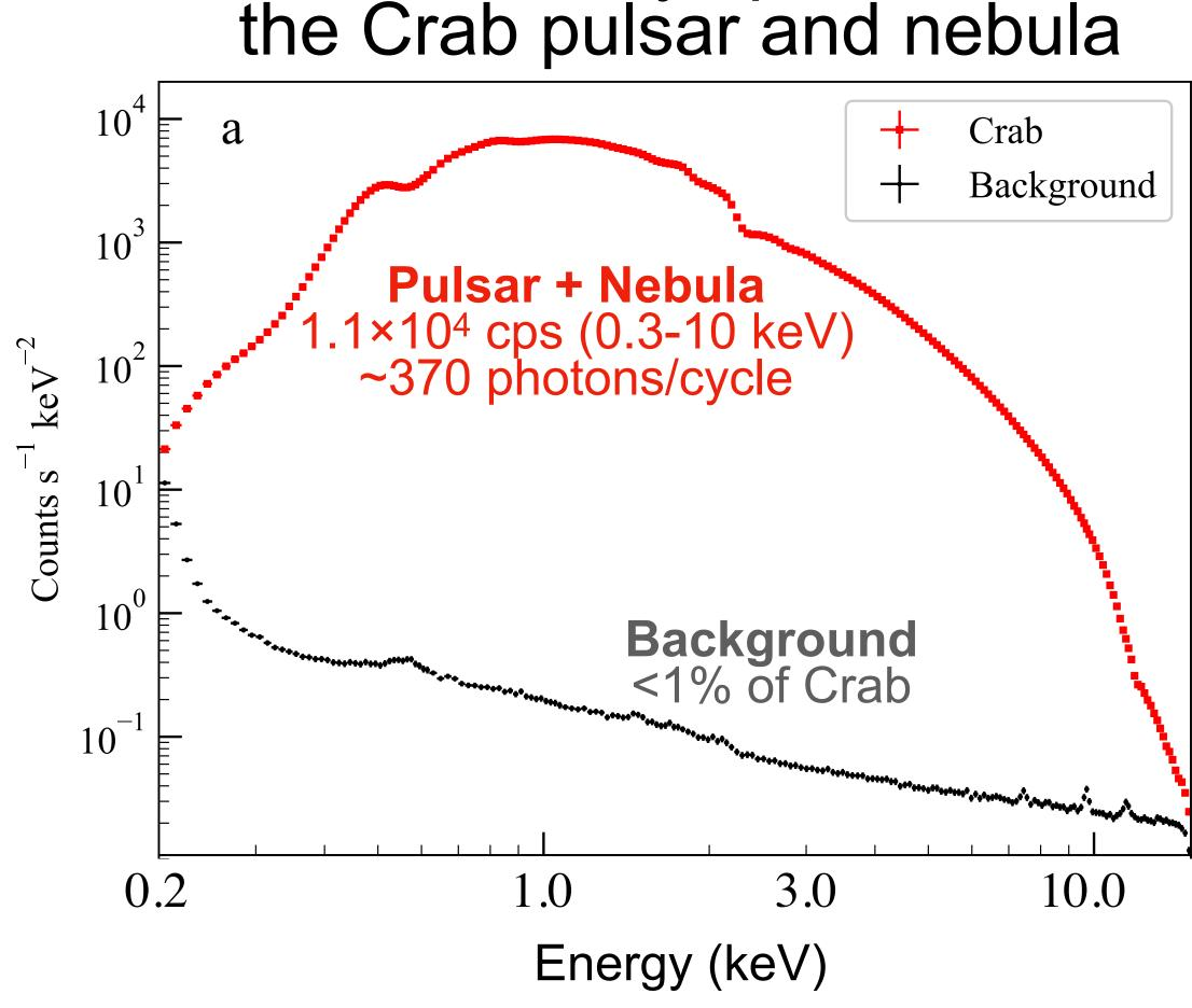
Pulse signals are detectable within 1 sec, ×50 larger photon statistics than Hitomi. Free from pileups, dead time, and data transfer loss (throughput 3.8×10<sup>4</sup> cps).
