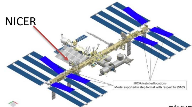
Figure 1. iROSA installed locations
