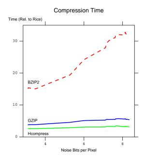
Fig. 3.— Image compression CPU times for Hcompress, GZIP, and BZIP2 relative to the compression time when using Rice, when using the default (row by row) image tiles.
