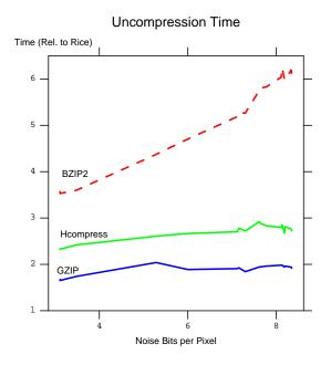
Fig. 4.— Image uncompression CPU times for Hcompress, GZIP, and BZIP2 relative to the uncompression time when using Rice, when using the default (row by row) image tiles.
