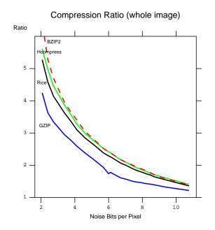
Fig. 2.— Compression ratios of the 4 algorithms when compressing the whole image as a single tile. BZIP2 now slightly exceeds the compression ratio of Hcompress for images with less than 5 bits of noise.
