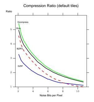
Fig. 1.— Compression ratios of the 4 algorithms when using the default image tiles. BZIP2 performs worse than H compress and Rice, but better than GZIP.
