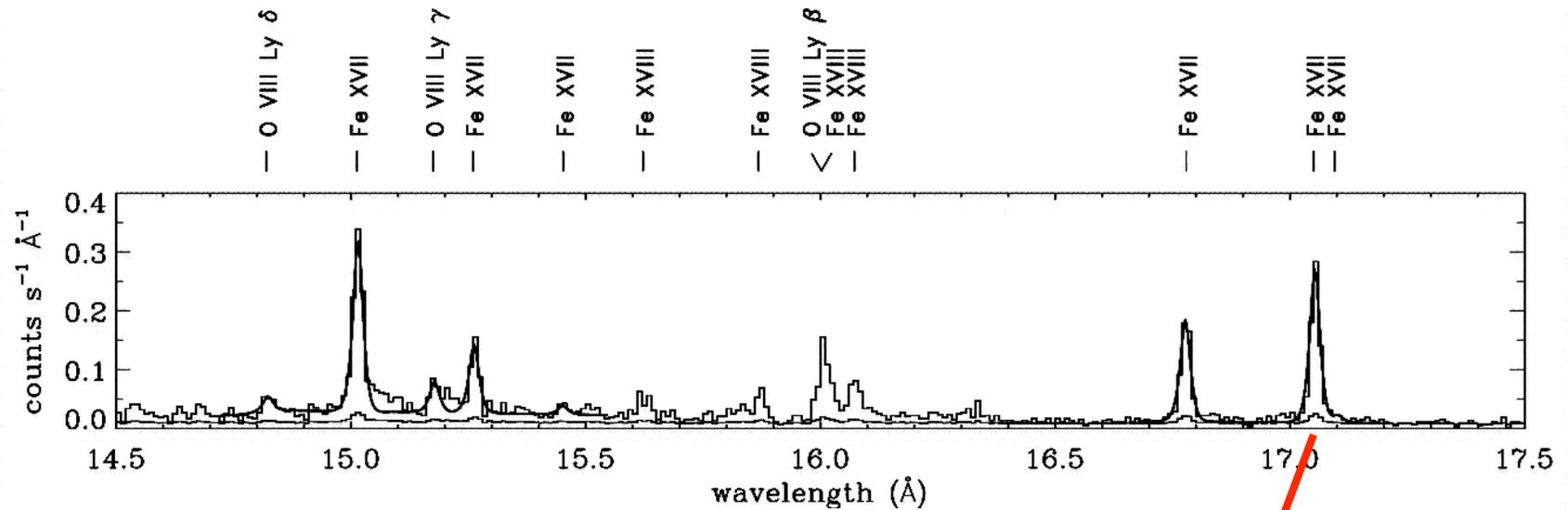
Here they have extracted the ratio of two very closely spaced Fe XVII lines, which are a density or a UV flux diagnostic
