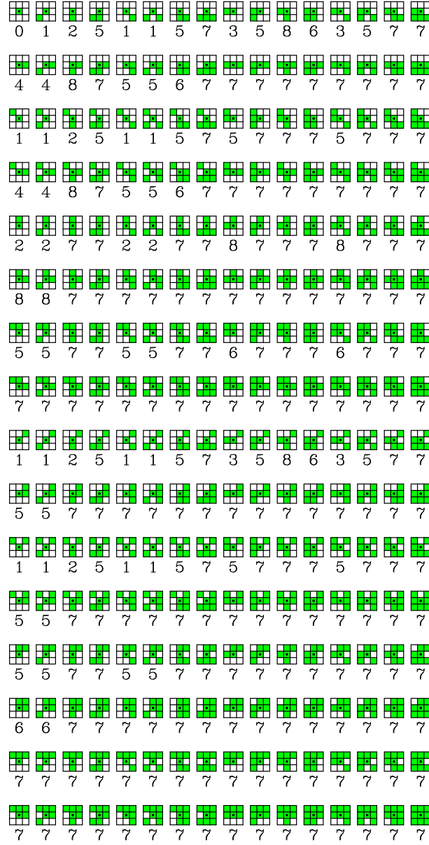
Figure 2. Schematic of all 256 possible 3x3 hit patterns with corresponding initial grades. Each grid shows a 3x3 pixel event island, with the readout node toward the lower left. Green pixels indicate a pulse-height greater than or equal to the split threshold, with the central pixel (with a dot) required to be a local maximum above the event threshold. The corresponding initial grade number (0–8) is shown below the 3x3 grid.
